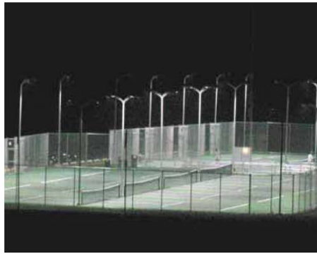
Full cutoff lighting produces more useable illumination.
