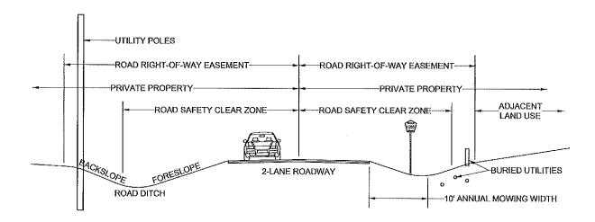
Safety is the primary goal of roadway design and maintenance. Safety is affected by pavement condition, road geometry, intersections and drainage. Safety is also affected by the condition of the adjacent roadside. The Federal Highway Administration recommends that new highways include a roadside clear zone free of obstacles, to increase visibility, and to provide space for errant vehicles to recover. The roadside clear zone concept is also applied to existing roadways as conditions allow.
